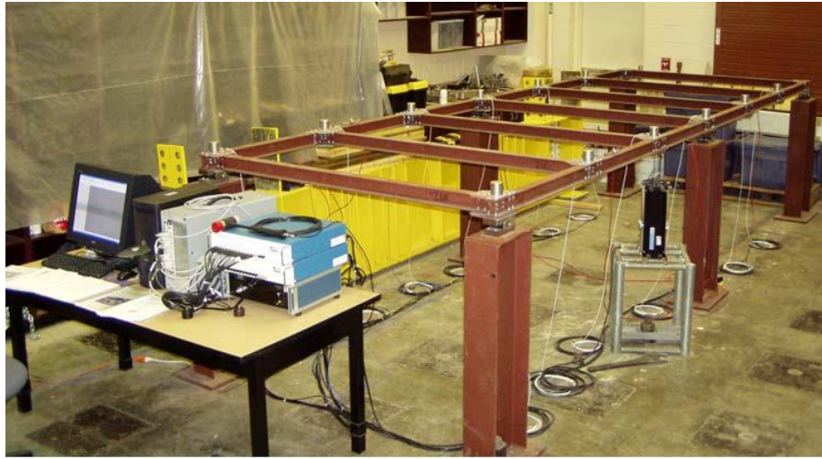
Figure 9: Two-Span Steel Grid benchmark [26]
