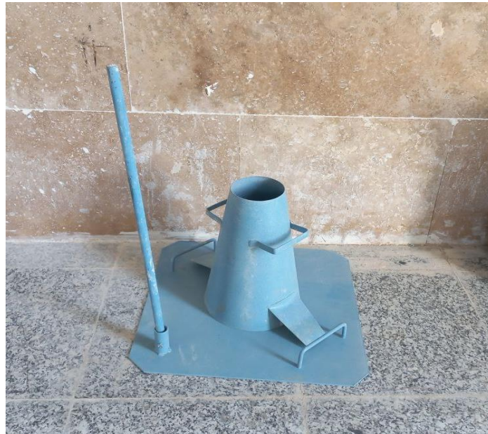
Figure 10. Slump test cone
