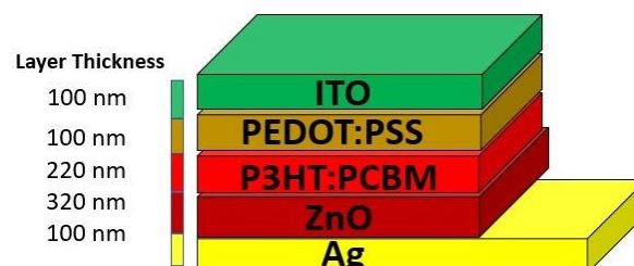
Fig. 11. Simulated Organic Solar cell with layer Thickness
