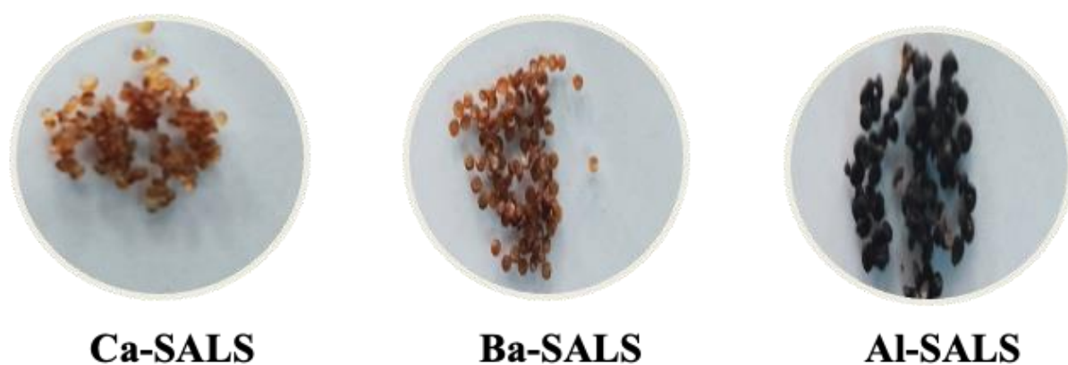
Fig. 2. Crosslinked HCQ drug-loaded SALS beads (dry)
