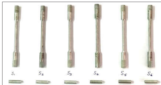
Fig. 3. Tensile and wear test samples
