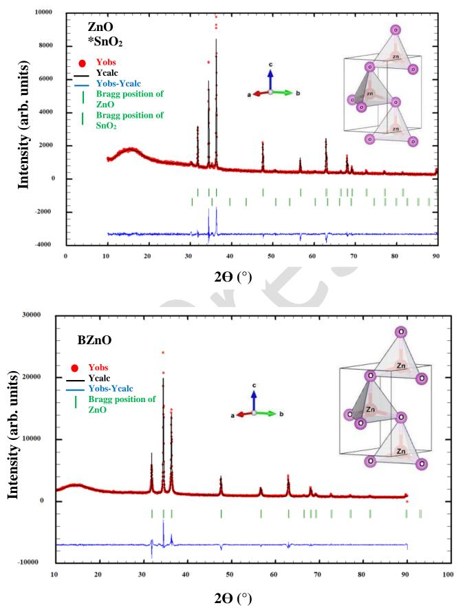
The good agreement between experimental and fitting diffraction lines ensures the hexagonal structure of ZnO and BZnO samples with a Space group P63mc and there are no signs of a
