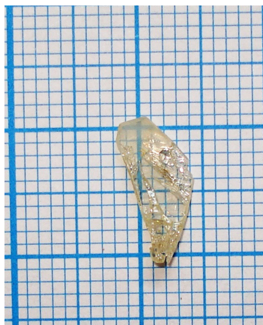
Fig.1. ZnS crystal grown at 1000 oC with \Delta T = 15 oC.
