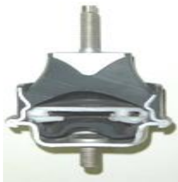
Fig24. Hydraulic engine mount with Inertia track
