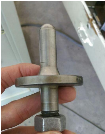
Fig2.Steel imp actor used in drop ball tests
