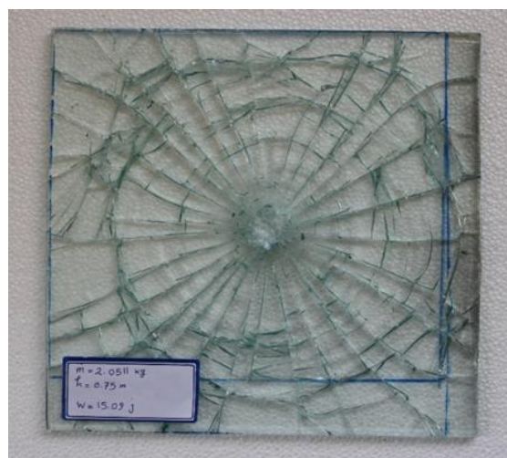
Fig12. .specimen after test code D-B-T-5
