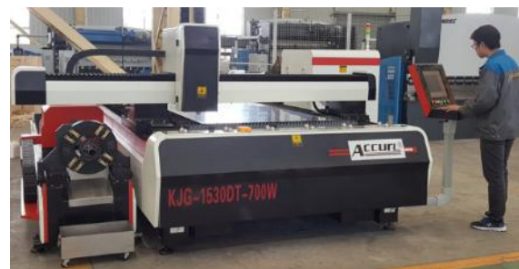
Figure 1: ACCURL laser tube cutting machine in operation
