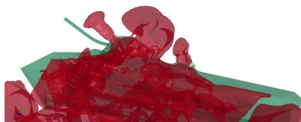
Fig.11. Transparency Schematic illustration of wave blast depression trough BTR-80 IFV.
