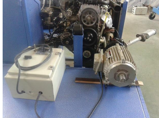
Figure 1: Motor setup, electric motor and inverter
