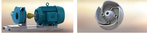
Figure 6: The view of the impeller and modeled pump along with the mounted drive
