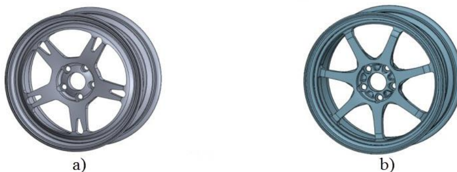
Figure 28: a) Optimized Wheel, b) Wheel in the market
