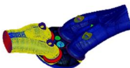
Fig. 1. the computational domain of the engine model
