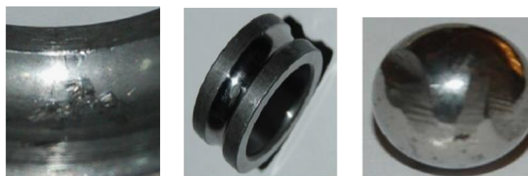
Fig2. Bearing component with fault (Shahrekord test rig), outer race fault, inner race fault and ball fault
