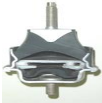
Fig24. Hydraulic engine mount with Inertia track
