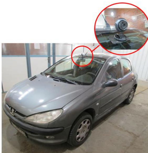
Fig7. Equipped trial car in AVCS Lab.
