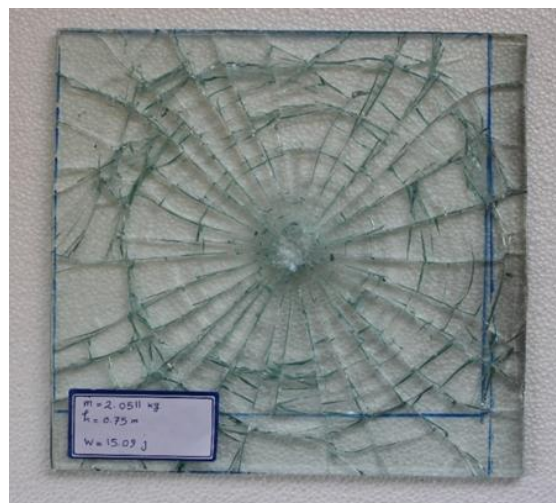
Fig12. .specimen after test code D-B-T-5
