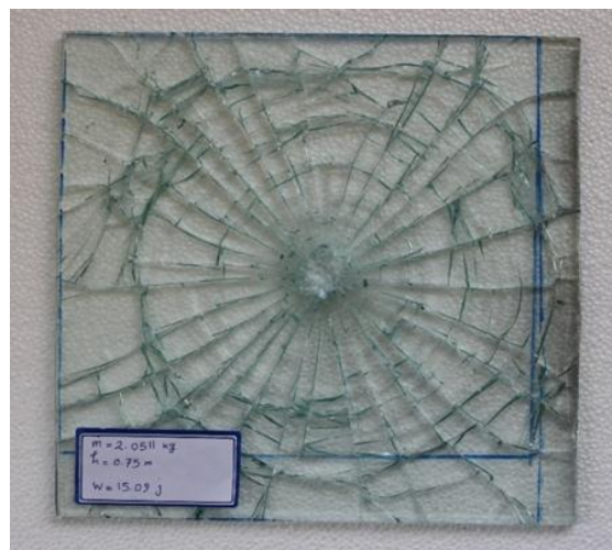
Fig12. .specimen after test code D-B-T-5
