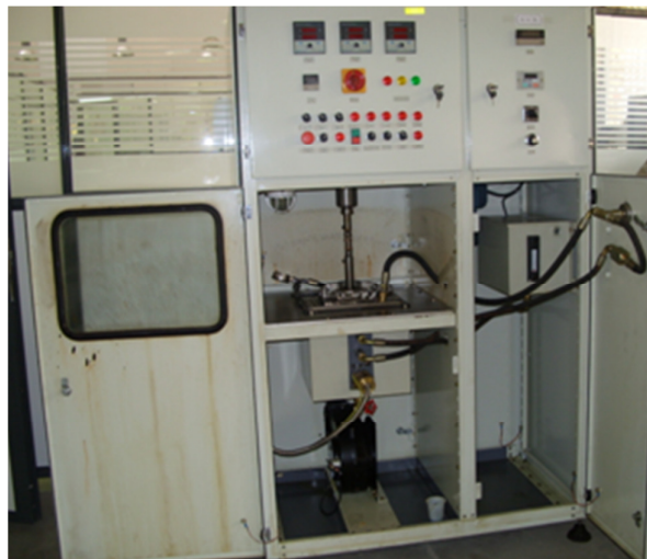
Fig16. Test setup of external gear pump
