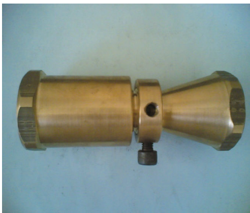
Fig. 13. Schematic of optimum venturi
