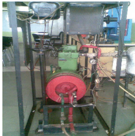
Plate 2. Rope Drake Dynamometer
