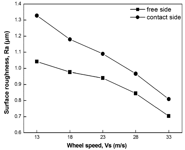
Fig. 5 Dependence of Surface roughness ( R_a ) on the wheel speed for the prepared FINEMET ribbons
