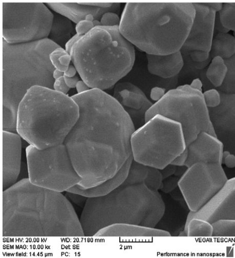
Fig. 1. SE-SEM micrograph of primary tungsten powder.
