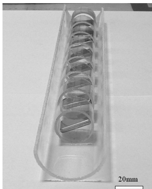
Figure 1. Test coupons in the quartz sample holders
